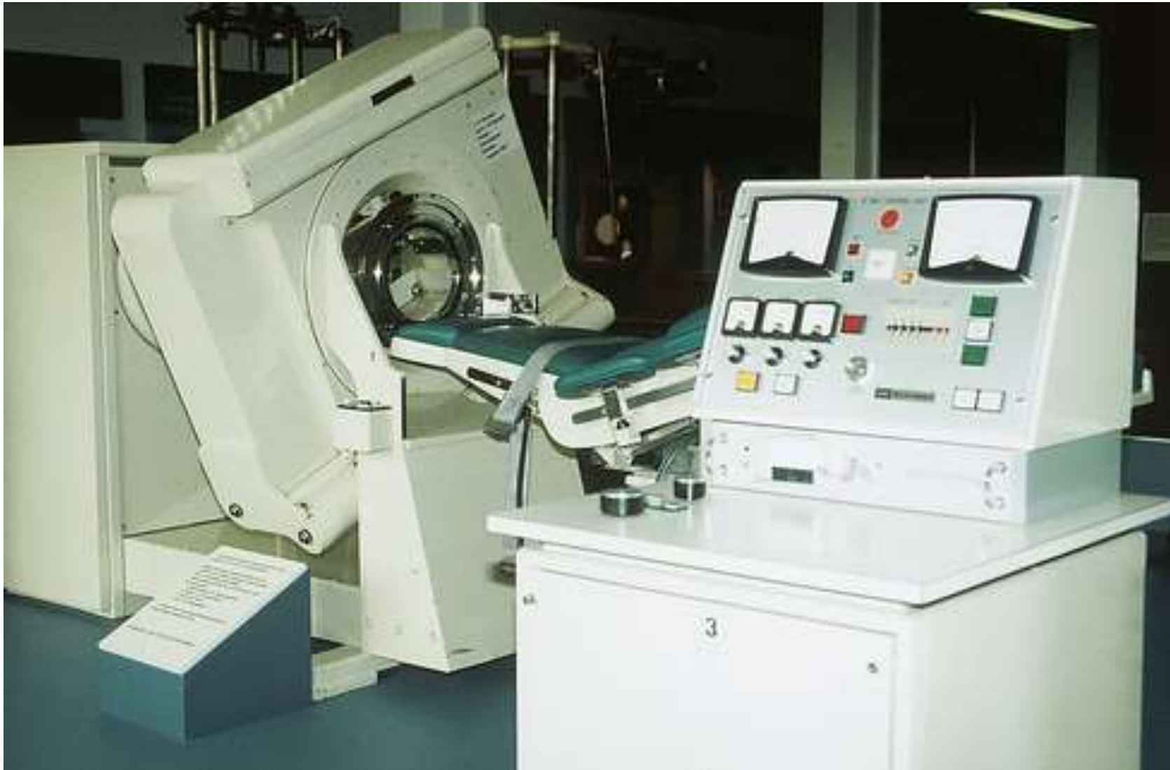
First-generation EMI CT unit: dedicated head scanner. (Photograph taken at Reöntgen Museum, Lennep, Germany.)
